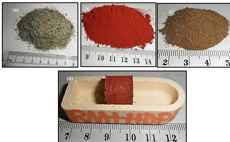
Fig. 3: (a) PWS, (b) iron oxide, (c) CNS (raw) and (d) cylindrical pellet of iron oxide-PWS
