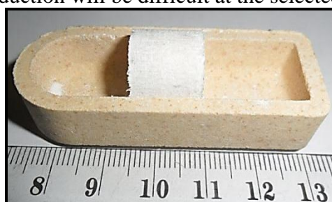
Fig. 2: Composite pellet (of Al_2O_3 + PWS) utilized for thermal decomposition of PWS at 1500 °C
