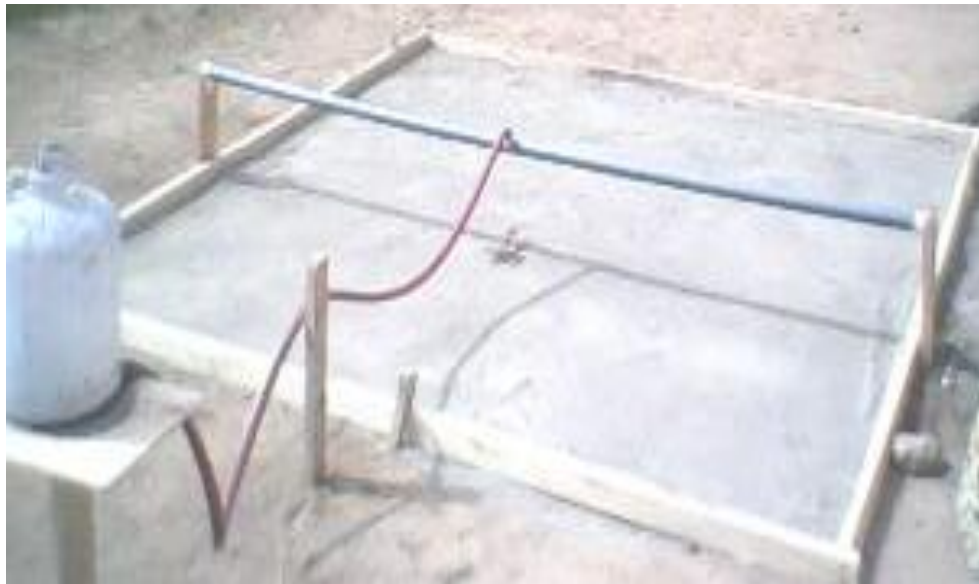
Figure 3: Experimental setup of soluble pollutant flow through fine sand.
