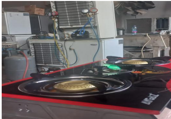
Figure 2: The Complete Setup of the LPG Refrigeration System
