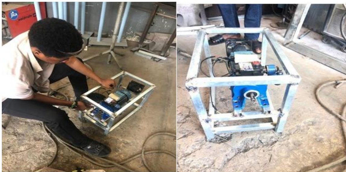
Figure 6: Assembled Prototype of the Oil Press Machine.
