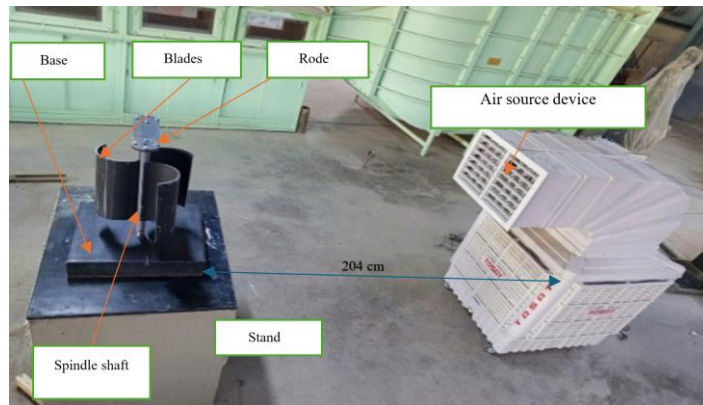
Plate 1: Current model of Savinuos VAWT (Experimental setup).
