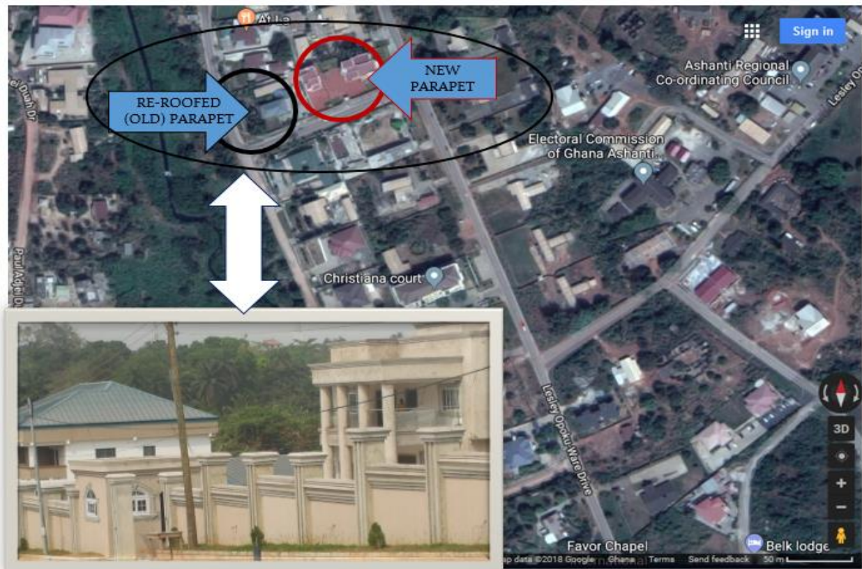
Fig. 2. Green re-roofed parapet building with a newly constructed concrete parapet roof next to each other off Lesley Opoku-Ware Drive. Source: (inset) Authors, 2016; Google maps, 2018.
