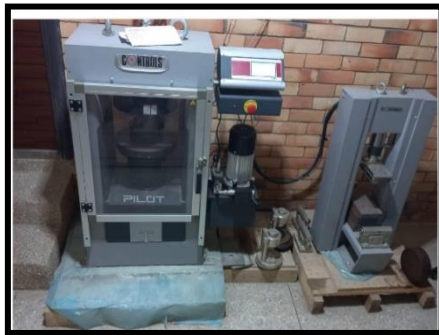
Figure 4: Versatile Automatic Pilot PRO compressive testing machine, at the Ghana Standard Authority Laboratories, Legon, Accra
