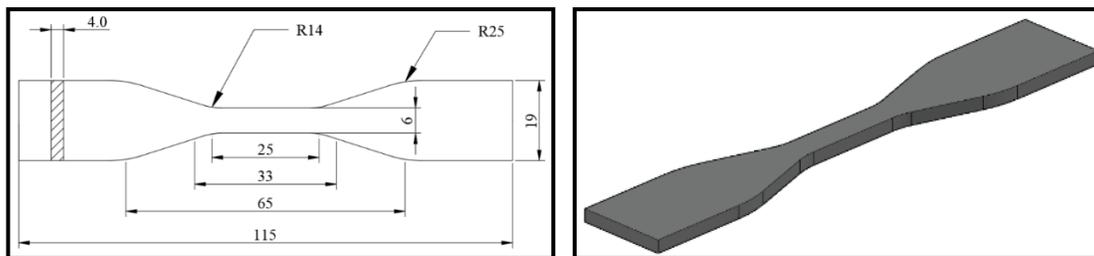
*Figure 2: ASTM D638 Type IV and modelled tensile specimen*
