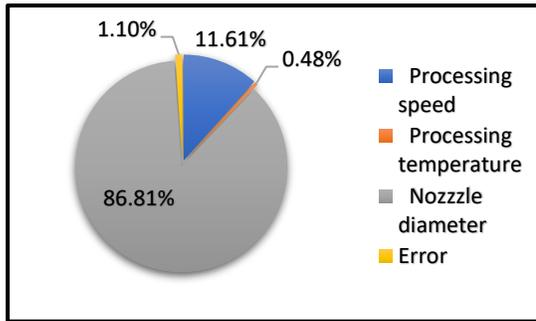
Figure 5: Significance of process parameters for Ultimate Tensile Strength
