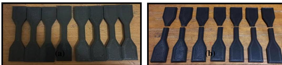
*Figure 3: Prepared PLA tensile test samples (a) PLA test samples before testing and (b) broken PLA test samples after tensile testing*
