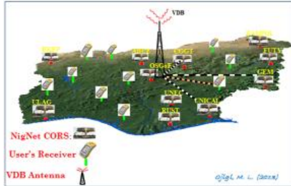
Fig.3.1: Centralized Network RTK data processing Model for Nigeria
