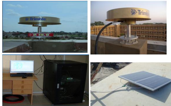
Figure 1.2: State-of-the-art GNSS CORS Equipments
