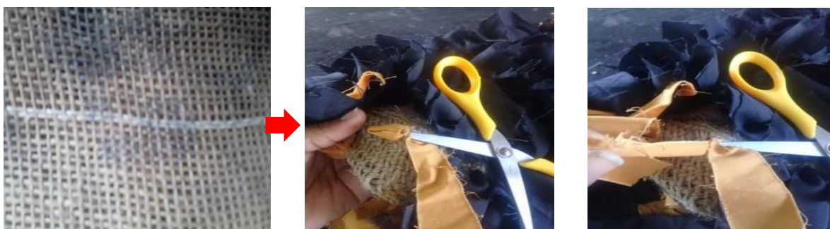
Plate 8: Cut out fabric pieces tuck-in through the porous of the jute material
