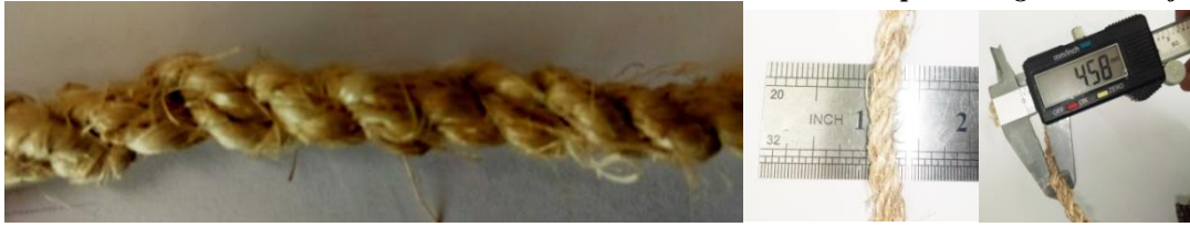
Figure 4: Twisted yarn and cord measurement
