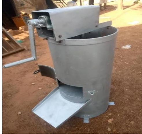
Figure 5: A Photograph Showing the Manufactured Groundnut Roasting Machine
