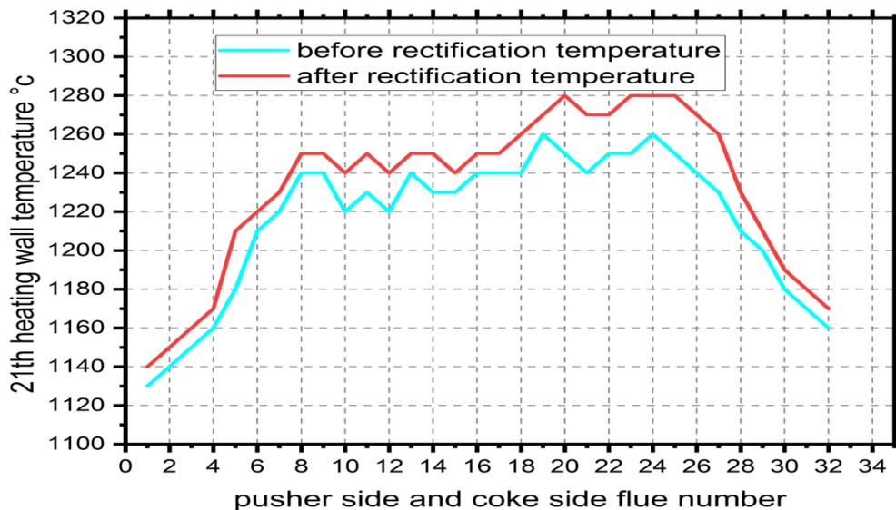
Figure 2: 50<sup>th</sup> heating chamber wall temperature with heating flue number
