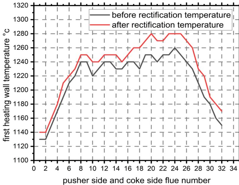
*Figure 1: Temperature fluctuation in the pusher and coke sides*
