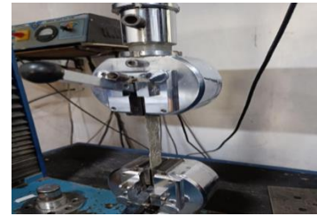
Plate 6: Strength of composite material using Universal Testing Machine
